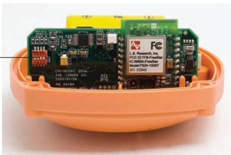
Figure 8: StatusCheck Dip Switch Location
