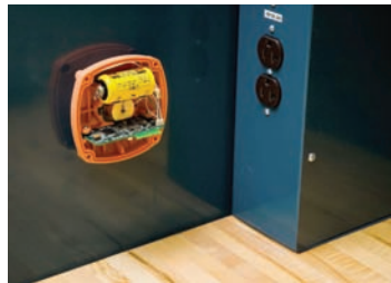
Figure 8.1: StatusCheck End Node Accelerometer Offset Adjustment Orientation
